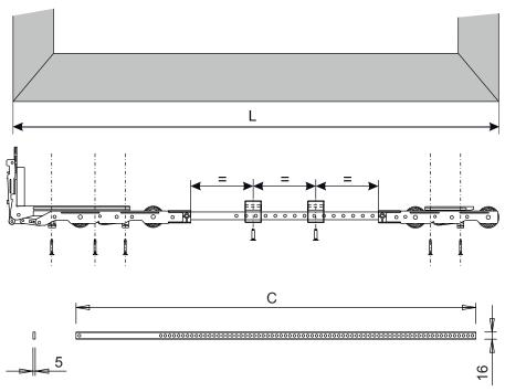
Rod to pulleys fixing
